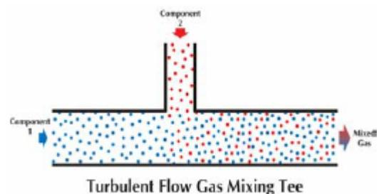
Producing gas mixtures in cylinders is normally accomplished by successively adding one component after another to the cylinder. This procedure produces layers of gases in the cylinder. After filling, the gases in the cylinder can be mixed by rolling the cylinder, or natural mixing between the gas layers will occur after some period of time, normally a matter of days or weeks. Use of a dip or distributor tube in the cylinder will dramatically improve mixing in the cylinder.
